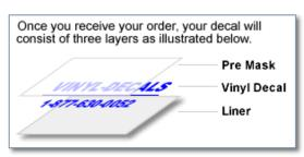
The top layer is called transfer tape or pre-mask. It looks somewhat like regular masking tape. The middle layer is the actual decal and this will come up with your transfer tape when you're ready to apply. The bottom layer is a backing paper with a waxy surface.
