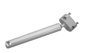
multi-unit rod holder. It is available in two different locking styles, bayonet and straight slotted (as shown to the left). A straight slot is recommended with flush mounts with drain hoses.
